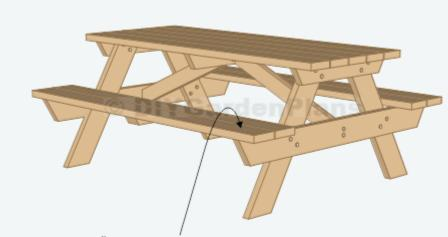
Screw 2  $1/2^{\prime\prime}$  deck screws through the seat and into the seat support.
