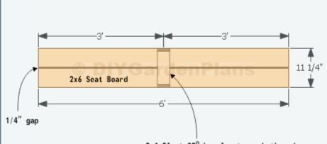
2x4 Cleat 30° bevel cuts on both ends.
